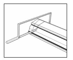
The gutters have to be cut in the correct length. PVC gutters can be cut easily with a small saw. Make sure the cut is straigth and clean. If necessary, you can clean the cut with a knife or a piece of sandpaper. Also wipe off remaining sawdust from the gutter.
