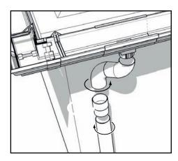
With elbows you can guide the downpipe from the gutter outlet to the wall. Connect the downpipe and elbow by using glue. Fix the pipe clips at a maximum of 2 meters. Push the pipe into the clips and close them.
