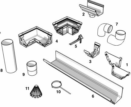
Determine the position of the outlet. That is automatically the lowest point. After that, you can also determine the highest point. Install a bracket at the lowest and one at the highest point. A string secured between both brackets will assist in installing the remaining brackets.
